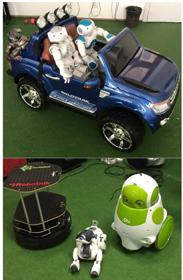
Fig. 3. Robotic hardware at CIT – top left to bottom right – AIBO, Nao V1, Nao V3 in customized sensor-enabled automobile, TurtleBot, another AIBO and Qbo.
