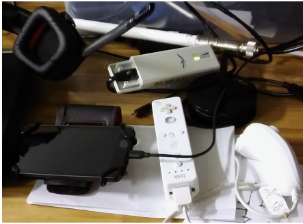
Fig. 5. Typical accessories used during SWAT trainings: Wiimote/Nunchuck, Android mobile device, external antenna system & headphones with microphone.
